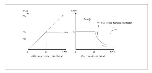
Fig. 3.1 Principle U/f characteristic and torque
