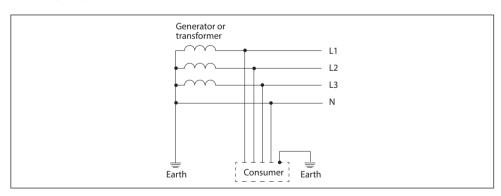
Fig. 6.4 TT system: Earthed neutral conductor and individual equipment/installation earthing
