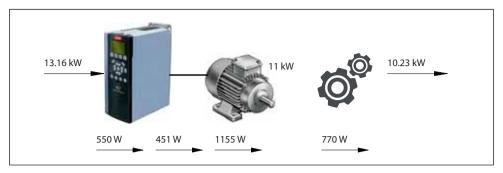
Fig. 4.20 System losses during motor operation
