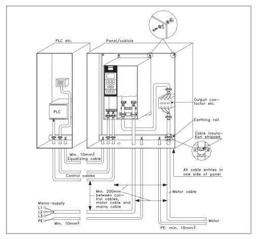
Fig. 5.10 Typical measures in practice in a simple frequency converter installation
