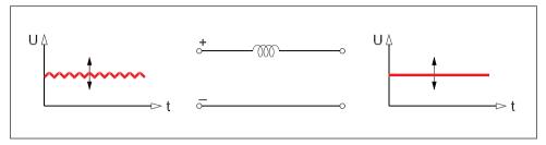
Fig. 2.8 Variable DC intermediate circuit
