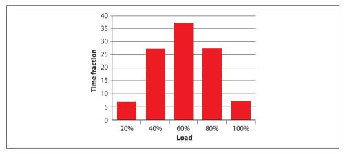
Fig. 4.13 Load over Time fraction diagram indicates how long a load is operated at part load
