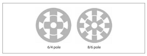
Fig. 1.33 Switched reluctance motor configuration examples
