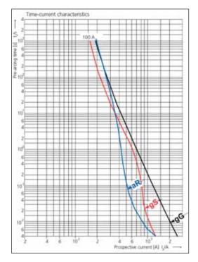
Fig. 6.9 Time-current characteristics of fuses
