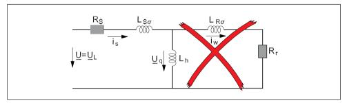
Fig. 2.25a Motor equivalent circuit diagram under "no-load"
