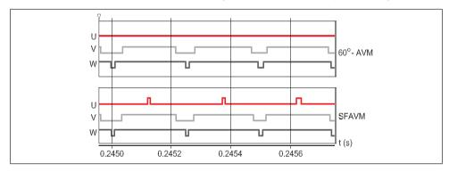
Fig. 2.18 Switching sequence of the 60° AVM and SFAVM methods for a number of 60° intervals
