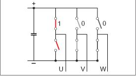
Fig. 2.15 Inverter switch states
