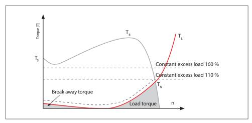
Fig. 9.3 Frequency converter with an optimised characteristic for quadratic loads and an over-load of 110%. In order to achieve higher breakaway torque, the drive is sometimes started with a constant torque before the quadratic characteristic is used
