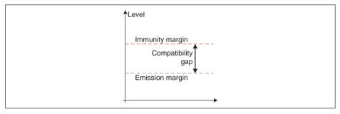
Fig. 5.2 Explanation of compatibility gap
