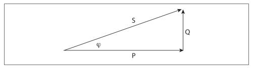
Fig. 7.2 Components of AC Power: Real Power (P), Reactive Power (Q) and Apparent Power (S)
