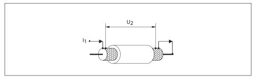
Fig. 5.6 Illustration of transfer impedance
