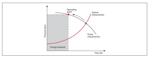
Fig. 4.14 Energy required in a variable torque pump application for throttle control
