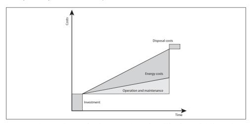
Fig. 4.17 Initial costs usually account for only approximately 10% of overall life cycle costs. The higher initial costs of an energy-saving device often pay for themselves in next to no time
