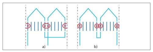
Fig. 1.4 Two coils in one phase connected in series to a) two poles b) four poles
