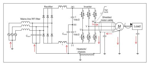
Fig. 5.4 Propagation of interference in a Frequency Converter
