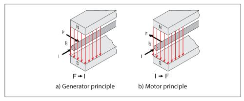
Fig. 1.3 Principle for electromagnetic induction
