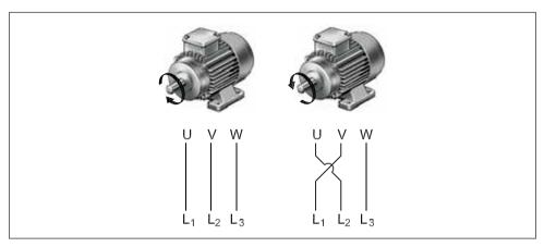
Fig. 3.6 The rotation direction of the motor reverses when the phase sequence is changed
