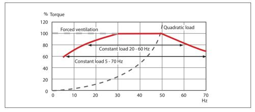
Fig. 9.4 Obtaining a good match in speed selection
