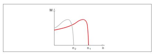
Fig. 1.17 Torque characteristics when changing pole number
