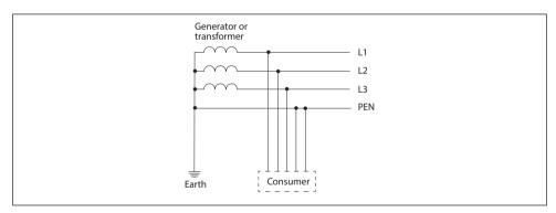
Fig. 6.2 TN-C system: In the entire system, the neutral conductor and the PE conductor are combined in the PEN conductor.
