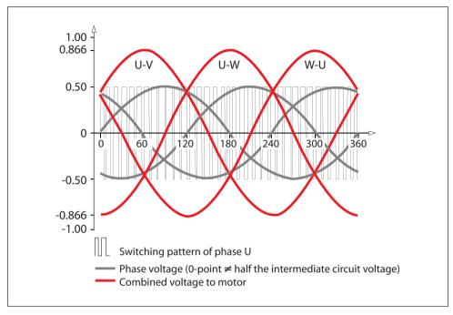
Fig. 2.14 Output voltage PWM
