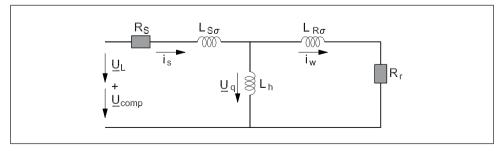
Fig. 2.25b Motor equivalent circuit diagram under "load"
