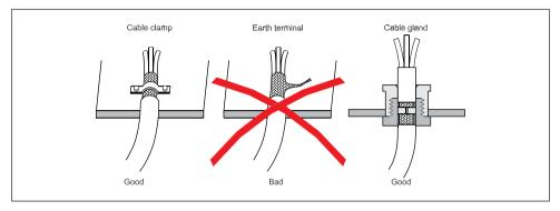
Fig. 5.8 Installation of cable shield
