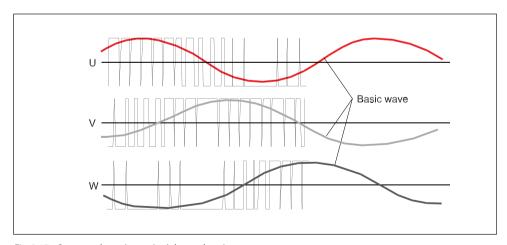
Fig. 2.17 Output voltage (motor) – (phase-phase).
