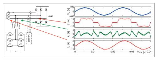
Fig. 7.6 Operation Principle of an Active Filter
