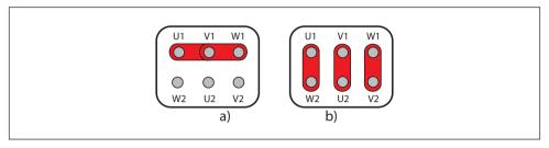
Fig. 1.20 Star (a) and delta (b) configuration of motors via jumpers on the terminal block
