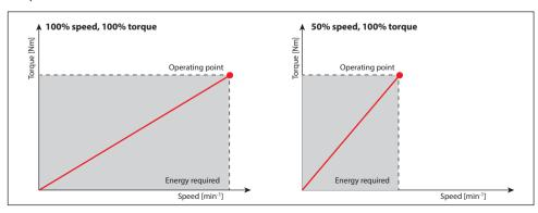
Fig. 4.16 Energy required at different speed and loads
