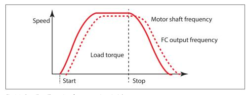
Fig. 9.6 Start/Stop illustrations for regenerative principle
