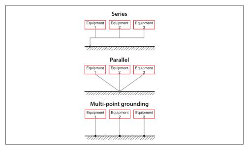
Fig. 5.5 Single point grounding in series or parallel and multi-point ground is possible
