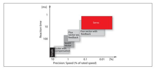
Fig. 2.20 Speed control performance control classification
