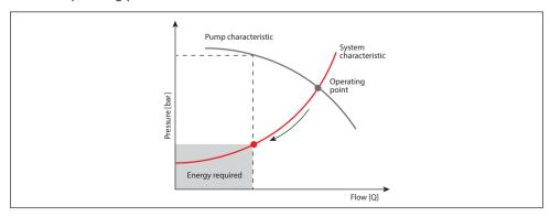
Fig. 4.15 Energy required in a variable torque pump application for speed control
