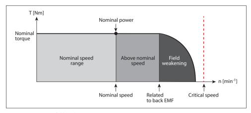
Fig. 1.25 Operation in field weakening area
