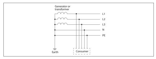
Fig. 6.1 TN-S system: Separate neutral and PE conductors.
