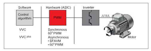
Fig 2.24 Basic principles of current standard frequency converters from Danfoss
