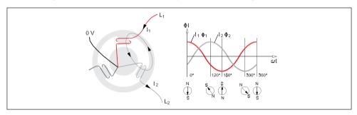
Fig. 1.8 Two phases produce an asymmetrical rotating field
