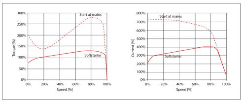
Fig. 4.9 Comparison motor start direct on mains with motor started by a softstarter (400% current limit)
