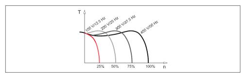
Fig. 1.18 Torque characteristics with voltage/frequency control
