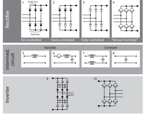
Fig. 2.3 Main component topologies
