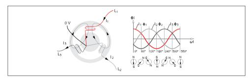
Fig. 1.9 Three phases produce a symmetrical rotating field
