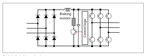
Fig. 3.11 Brake "chopper" and resistor
