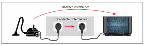
Fig. 5.1 Difference between radiated and conducted interference
