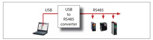
Fig. 8.6 USB to RS 485 communication
