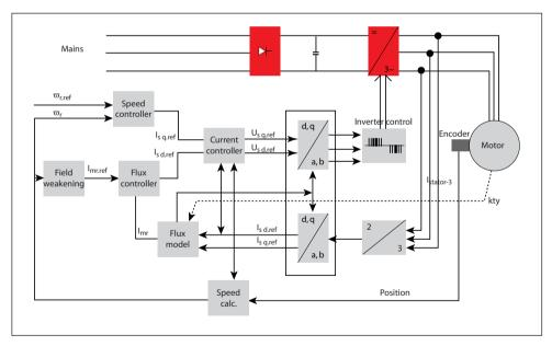
Fig. 2.23 Structure closed loop flux vector control
