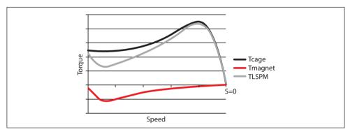
Fig. 1.27 Starting torque of LSMP is reduced compared to the pure squirrel cage torque
