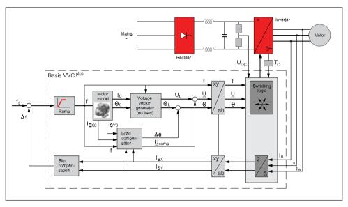
Fig. 2.26 Basic principles of Danfoss VVCplus control
