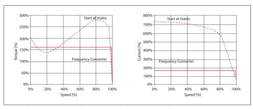
Fig. 4.10 Comparison motor start direct on mains with a motor started by a frequency converter at 160% overload
