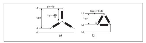
Fig. 1.21 Current and voltage distribution in star (a) and delta (b) configuration
