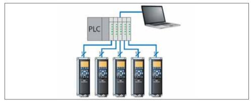
Fig. 8.7 Traditional wiring. No fieldbus
