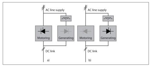
Fig. 3.12 Regenerative braking unit: motoring phase control on (a), motoring phase off (b)
