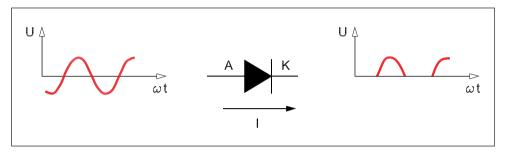
Fig. 2.4 How diodes work
