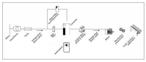
Fig. 4.18 Overview of motor drive system with various accessories
