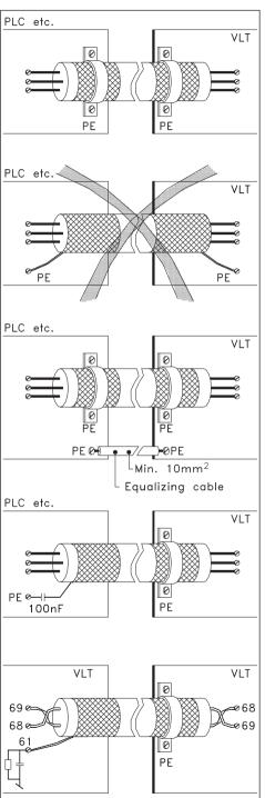
Control cables and serial communication cables should normally be grounded at both ends.
