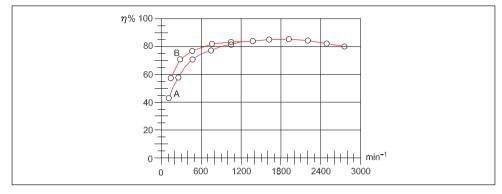
Fig. 4.4 Efficiency example of a frequency converter and motor combination
