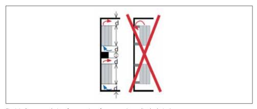
Fig. 9.9 Recommendations for mounting of converters (centralised solution)
