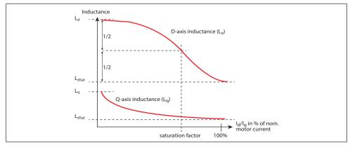
Fig. 1.32 Example of  $L_d/L_q$  relationship to  $I_d/I_q$
