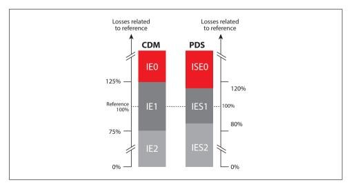
Fig. 4.7 Definition of CDM and PDS efficiency classes
