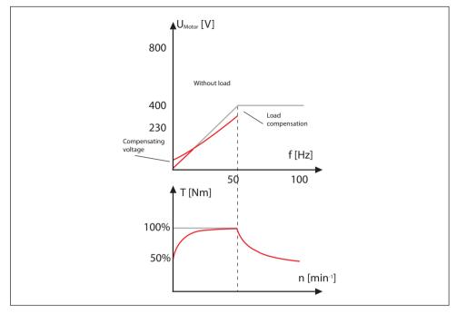
Fig. 3.3 Real U/f and T/n characteristic
