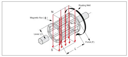
Fig. 1.11 Operational field and squirrel-cage rotor
