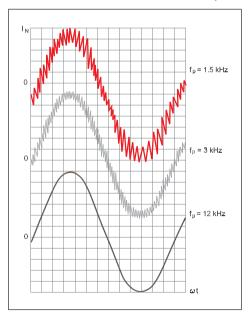
Fig. 2.12 Effect of switching frequency on motor current
