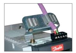
Fig. 8.5 Fieldbus connection
