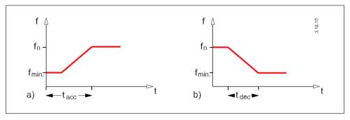
Fig. 3.8 Acceleration and deceleration times
