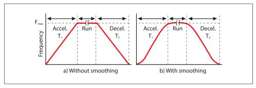
Fig. 3.9 Linear ramp a) and S-ramp (b)
