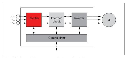
Fig. 2.2. Block diagram of a frequency converter with an intermediate circuit
