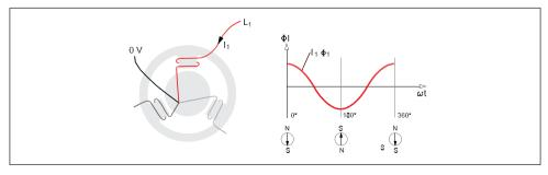
Fig. 1.7 One phase produces an alternating field
