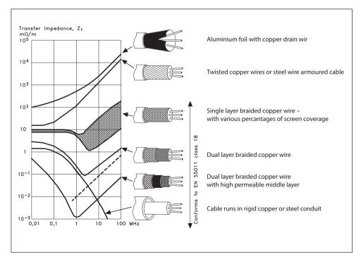
Fig. 5.7 Shielding performance of different cable types
