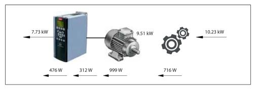
Fig. 4.21 System losses at regenerative operation
