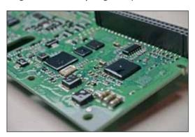
Fig. 9.8 Printed circuit board with conformal coated
