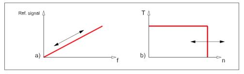
Fig. 3.4 Reference signal and motor torque relation
