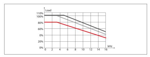
Fig. 9.5 Power reduction diagram for switching frequency and temperature
