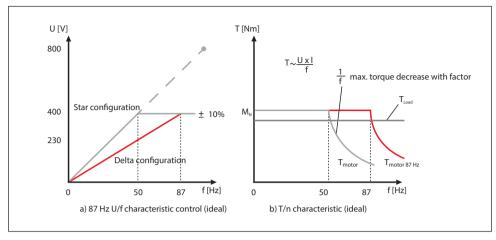
Fig. 3.2 87 Hz characteristic
