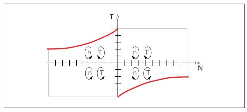
Fig. 3.7 Braking torque of the frequency converter during reversing
