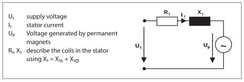
Fig. 1.23 Simplified PM motor equivalent circuit diagram
