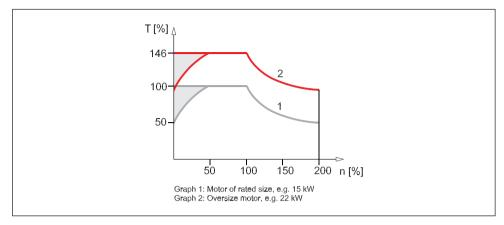
Fig. 3.13 T/N characteristics with and w/o external cooling
