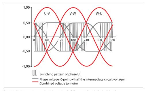
Fig. 2.16 With the synchronous 60° PWM principle the full output voltage is obtained directly
