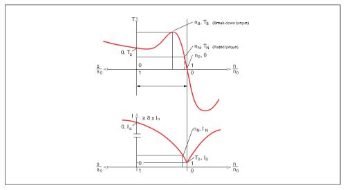
Fig. 1.14 Principal motor current and torque characteristics
