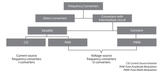
Fig. 2.1 Overview of frequency converter types
