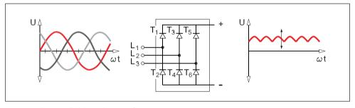
Fig. 2.7 Fully-controlled three-phase rectifier
