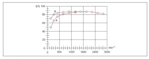
Fig. 4.3 Efficiency example of a 2-pole motor
