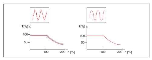
Fig. 3.14 Maximum continues torque and current shape relation
