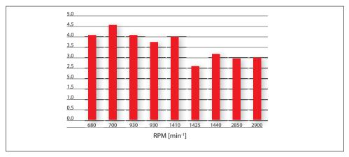
Fig. 9.1 Nominal current for 1.50kW motors of different poles and manufacturer
