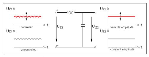
Fig. 2.11 Constant DC intermediate circuit
