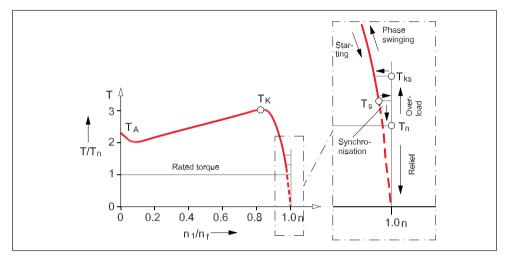
Fig. 1.30 Torque characteristic of a reluctance motor
