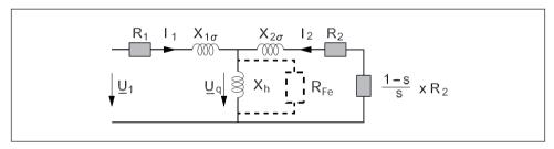
Fig. 1.15 Equivalent circuit diagram (one phase) for a motor operating under load
