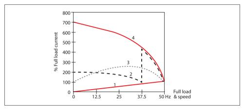
Fig. 4.8 Typical motors currents curves started by (1): Frequency converter at VT load (2): star-delta starter (3): Softstarter (4): direct on line (DOL)
