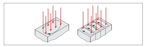
Fig. 1.6 Eddy-currents are reduced by the laminated form of the motor core
