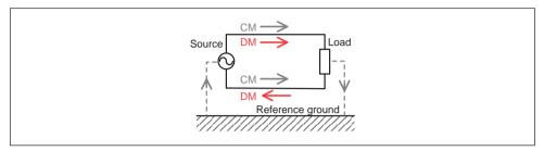
Fig. 5.3 Common-mode and differential-mode
