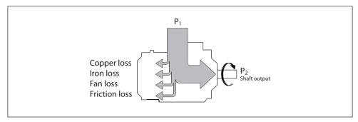
Fig. 1.5 Typical losses in the motor
