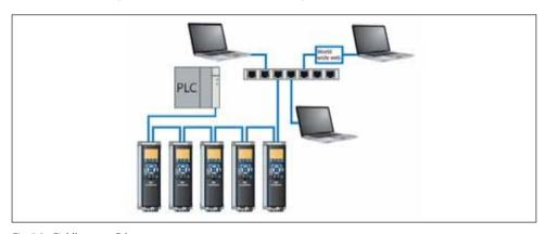
Fig. 8.9 Fieldbus over Ethernet
