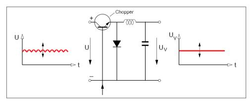
Fig. 2.9 Variable DC voltage intermediate circuit
