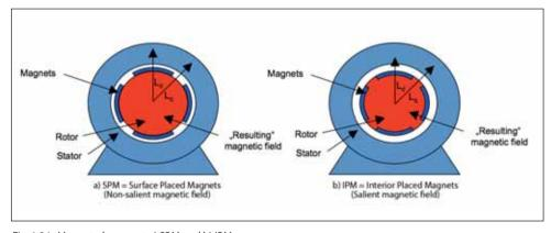
Fig. 1.24 Magnet placement a) SPM and b) IPM
