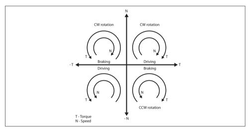
Fig. 3.10 Four Quadrant operation: Clockwise (CW) and Counter Clockwise (CCW)
