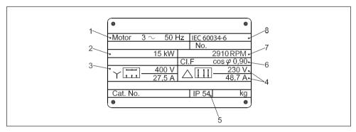
Fig. 1.19 Motor nameplate shows essential data
