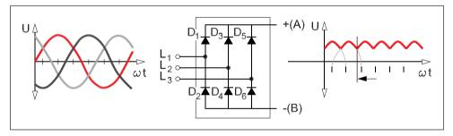
Fig. 2.5 Uncontrolled rectifier (B6-diode bridge)
