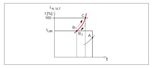
Fig. 3.5 Relation current limit and over current limit
