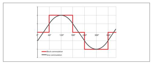
Fig. 4.11 Block vs. Sine-wave commutation
