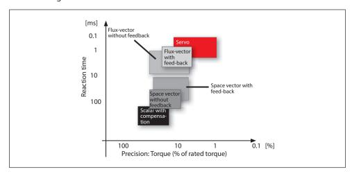
Fig. 2.21 Torque performance control classification
