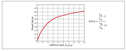
Fig. 1.28 Maximum power factor vs. saliency ratio
