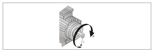
Fig. 1.13 Torque on the motor shaft is the force (F) x radius (r)
