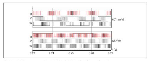
Fig. 2.19 Switching sequence of the 60° AVM and SFAVM methods for several periods
