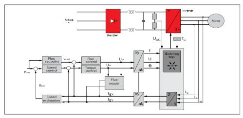
Fig. 2.27 Basic principles of Danfoss Flux Vector control
