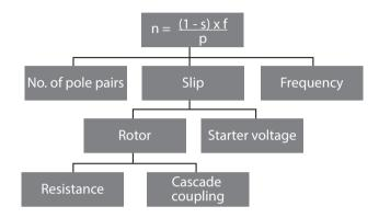
Fig. 1.16 Different options for changing the motor speed
